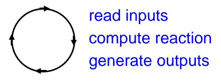
Synchronous = Zero-delay = within the same cycle parallel propagation of control parallel propagation of signals
