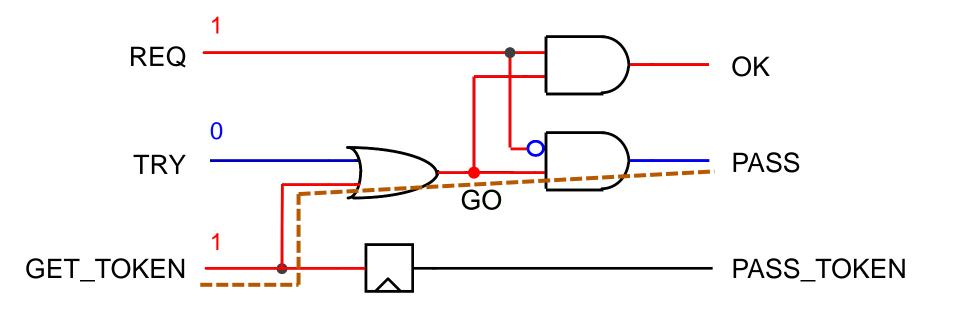
Since the network is acyclic, outputs stabilize in bounded time if inputs are kept constant Stabilization time is determined by the critical path
