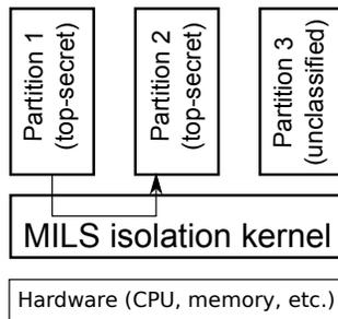
Fig. 3. MILS execution platform layers
