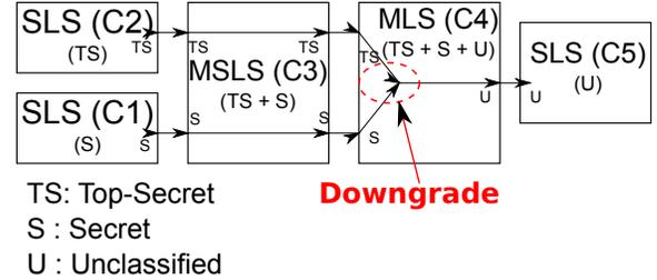
Fig. 2. Example of a MILS architecture
