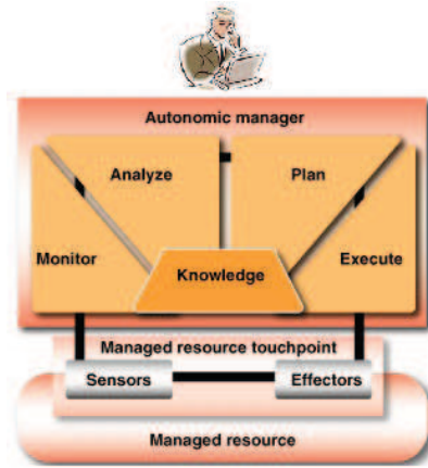
Figure 2.1: IBM's MAPE-K reference model for the ACL
