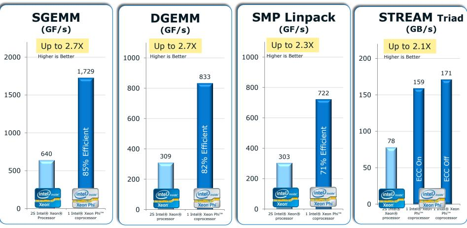
Coprocessor results: Benchmark run 100% on coprocessor, no help from Intel® Xeon® processor host (aka native)
